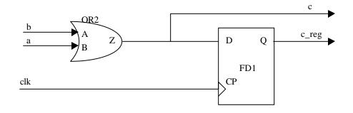
Since this netlist also represents the design, one can run the functional verification tests againts this netlist also. What is more important is the Static Timing Analysis (STA) on the netlist. STA reveals any potential timing problems like a setup or hold violation in the design. If there are some timing errors, those have to be fixed. A great deal of STA is explanined in the article released in July`99 issue-1.
